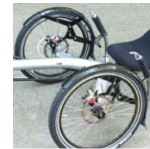
ABOVE: the optional front mudguards attach via the brake mounts.
